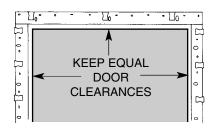
4. Hang the door. To align the frame and door, first close the door. Then begin with the header, using a screwdriver inserted in the alignment slot closest to the strike jamb. Create an equal gap between door and frame, and fasten the header above the strike jamb and the remainder of the header at every clip on the door side only.
