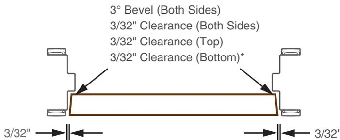
\*Additional clearance is required for Thresholds and various floor conditions.
